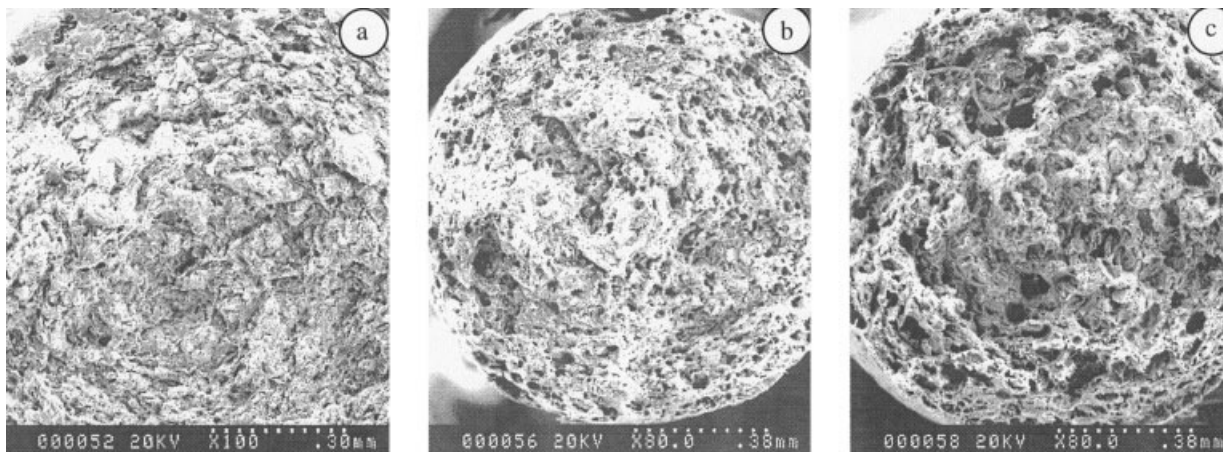
Figure 3 Effects of barrel temperature on the cell morphology of HDPE/WF foams. T_v = 160^\circ\text{C} , T_d = 140^\circ\text{C} . (a) T_b = 145^\circ\text{C} ; (b) T_b = 165^\circ\text{C} ; (c) T_b = 175^\circ\text{C} .
